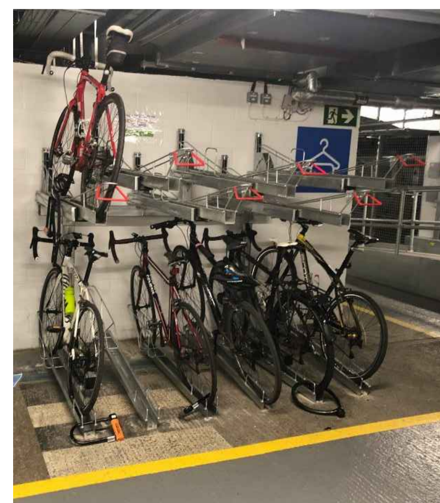
TWO TIER BICYCLE RACK FIGURE N.T.S. @ A1
